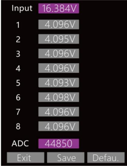
Measure the voltage of a fully-charged battery pack using a multimeter. Use the roller to select Input, then scroll until the value matches what was measured on the multimeter. Scroll down to save and press down on the roller to save. Repeat this process for each individual cell if needed. When finished, scroll to the exit option and press down on the roller to finish the calibration.
